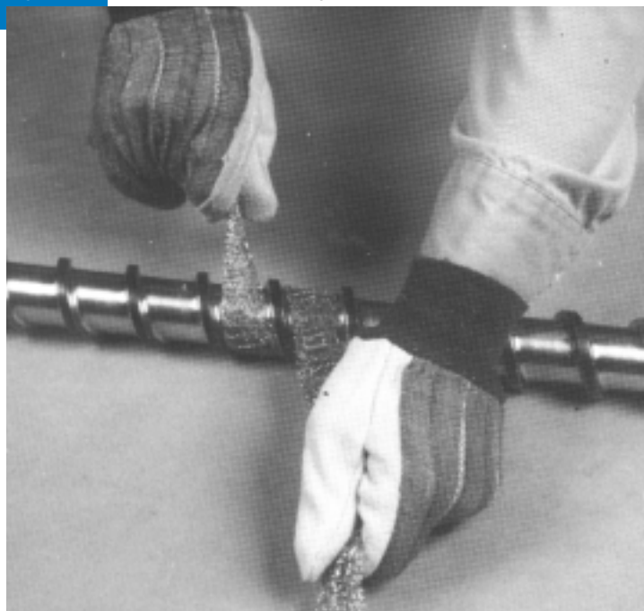
Figure 18 Mechanical Cleaning of the Screw
